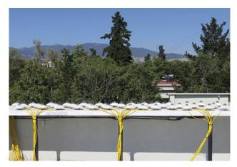
CMP 11 field pyranometers for AWS being calibrated at UNAM
