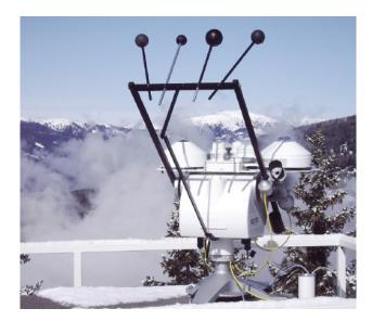
As part of the Austrian UV measurement network the SOLYS 2 also carries two UVS-AB-T radiometers, for global and diffuse UVA and UVB. In addition there is a CSD 3 sunshine duration sensor.
