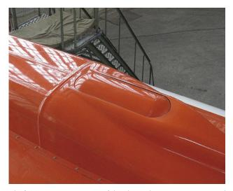
The fairing structure on top of the plane where CMP22, CRG4 and UVS-B-T radiometers are installed. (Photo: Roshydromet)
