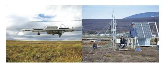
Left: CNR 4 Net Radiometer on support cables at Toolik Lake, Alaska
