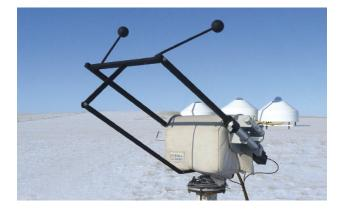
The trackers are fitted with CHP 1 pyrheliometers, CMP pyranometers and CGR 4 pyrgeometers; to measure direct, diffuse and global short-wave radiation and downwards long-wave radiation. An additional pyranometer and pyrgeometers measure reflected short-wave radiation and upwards long-wave radiation. All the pyranometers and pyrgeometers are fitted with CVF 3 ventilation units.
