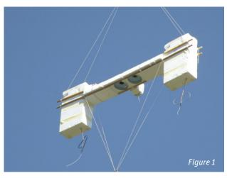
CNR 4 mounted between two Meteolabor radiosonde packages
