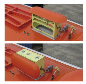
*View with fairing removed: rack with radiometers and the retractable cover. (Photo: Roshydromet)*
