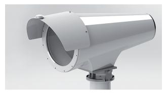
The scintillometer on its own measures changes in refractive index of the atmosphere, Cn<sup>2</sup>, but with the optional meteorological sensor kit it can calculate sensible heat flux. This kit consists of wind speed, temperature and pressure sensors and plugs directly into the X-LAS MkII receiver.
