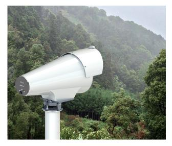
Fast, light and stable carbon fibre scintillometer for landscape scale flux measurements
