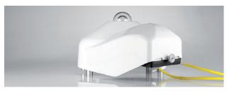
The CVF4 Ventilation Unit is specifically designed for the CMP Pyranometers and the CGR 4 Pyrgeometer. The Ventilation Unit is mounted to the Sun Tracker and then the radiometer is mounted on the CVF4 base plate. After levelling, the cover is fitted.
