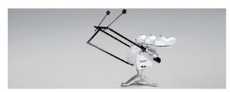
Where the conditions are less extreme, the SOLYS 2 sun tracker can be used. This has mountings for one pyrheliometer, a similar Shading Ball Assembly to the 2AP and an optional Sun Sensor. There are mounting kits for a second pyrheliometer or an Absolute Cavity Radiometer.
