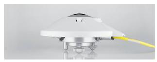
The CGR 4 Pyrgeometer meets all the requirements of BSRN and has the convenient design features of the CMP 21 and CMP 22. CGR 4 has a specially designed Silicon meniscus dome with an internal solar-blind optical filter coating and an external hard-carbon (synthetic diamond) coating. The unique thermal coupling of the dome to the housing provides the lowest thermal offsets available and no dome temperature measurement or correction is necessary.
