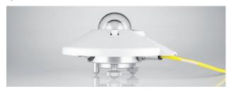
The CMP 21 and CMP 22 Pyranometers meet all the requirements of BSRN. They have high quality waterproof connectors for ease of exchange and calibration. The desiccant cartridge can be simply unscrewed and the highly accurate bubble level can be seen without removing the clip-on sun shield.
