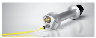
The CHP 1 Pyrheliometer meets all the requirements of BSRN. It has a quartz window to provide the required spectral response range and a double-tube construction to minimise the thermal shock effects of wind and rain. There are integrated alignment aids.
