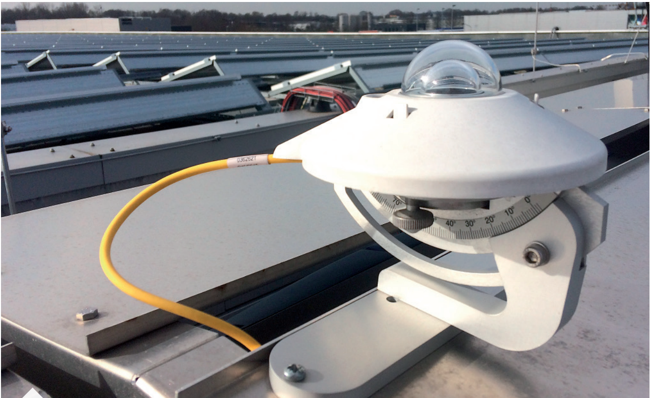
A tilted pyranometer on a roof in Etten-Leur, the Netherlands, a project of SolarAccess Sustainable Energy B.V.
