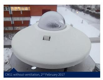
All the ventilation units performed well in keeping the domes clean and preventing the main effects of bad weather on the radiation measurements. There was an example in February of frozen sleet when all ventilation units successfully evaporated the accumulated sleet on the domes.
