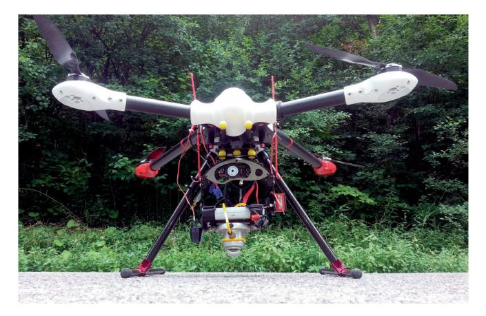
using Kipp & Zonen CMP6 and CMP3 pyranometers. The incoming global short-wave radiation was measured by the CMP6, mounted at the top of a 9 m telescopic mast and recorded by a Kipp & Zonen METEON data logger. The downward facing CMP3 was secured to the underside of a custom-made UAV, levelled by a motorized gimble, and the data recorded by another METEON.
