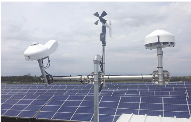
An automated weather station for solar farm performance monitoring. This turnkey system was customized by Campbell Scientific to meet the specific requirements for Ontario solar farms.
