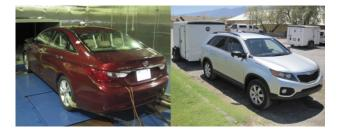
The Vehicle Evaluation Thermal Systems Group uses CMP 3 pyranometers to evaluate HVAC (heating, ventilation and air conditioning) and engine cooling systems in field tests in both desert and winter conditions. This way they ensure that vehicle systems respond as expected under the various sun load conditions that the North American climate offers. Pyranometers are used to measure the solar load at the roof
