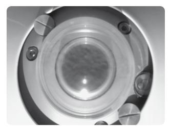
Pyranometer dome before cleaning
