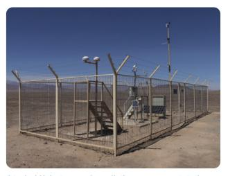
A typical Mainstream solar radiation measurement station
