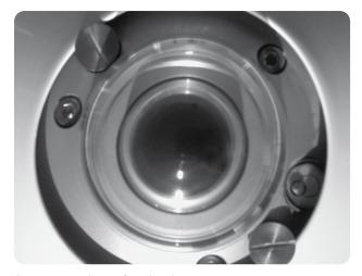
Pyranometer dome after cleaning
