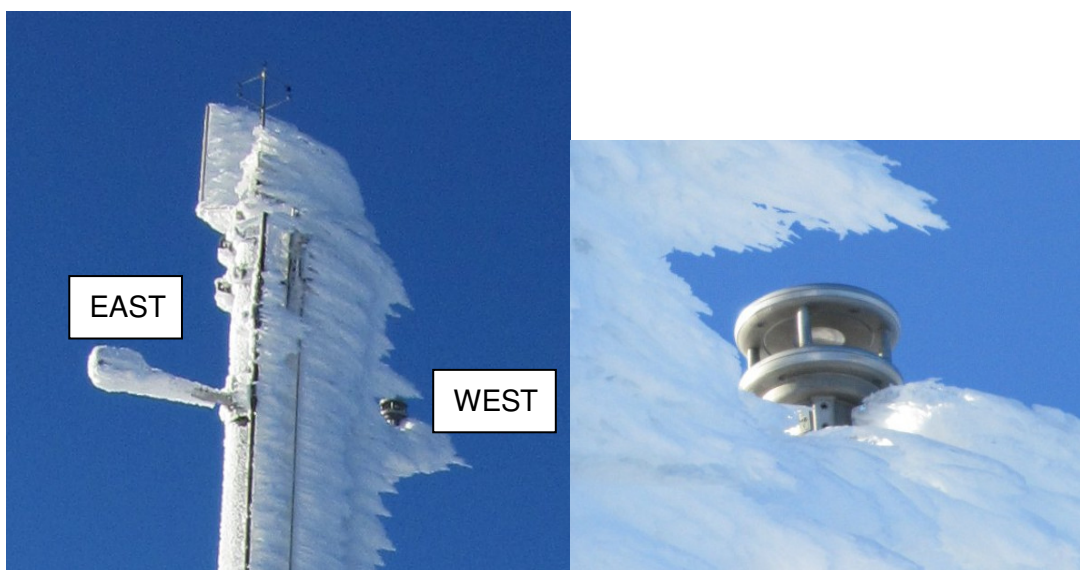
Figure 9: Left: Top of mast during a heavy icing event on 10.1.2012. Right: Zoom on Ventus wind sensor.
