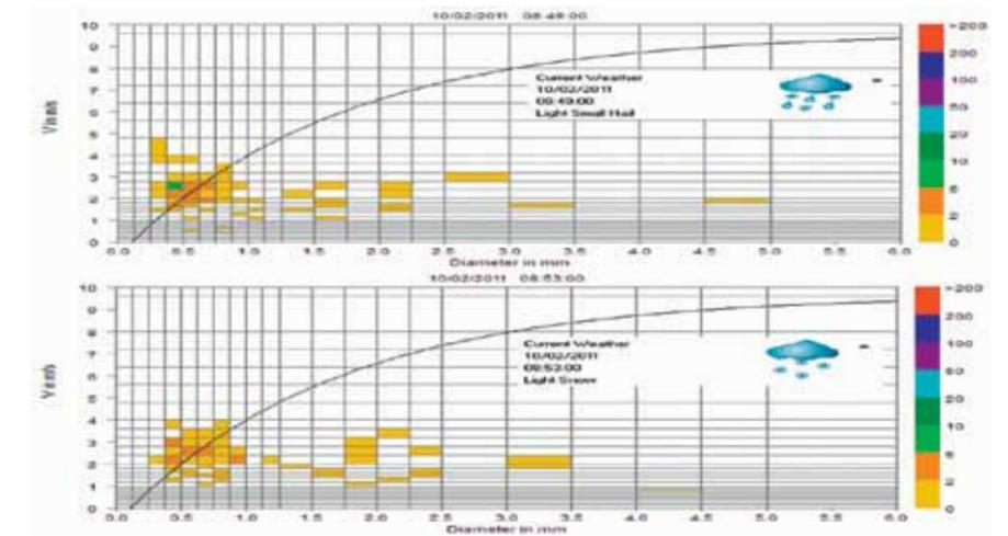
Displays of raw data spectra, showing Gunn-Kinzer line and automatic PW code (above “Light small hail”; below “Light snow”). The color code indicates the frequency of measured hydrometeors
