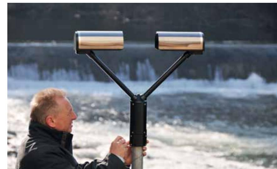
Figure 1: New laser-based disdrometer OTT Parsivel<sup>2</sup>
